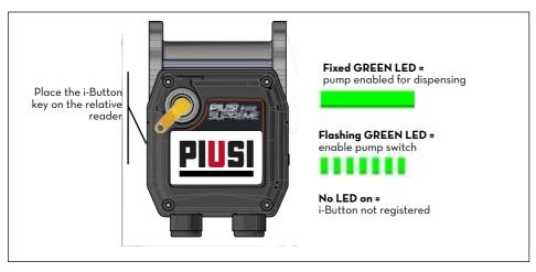
At the end of dispensing, the controller will return to the initial state, with both LEDs off, and will be ready to dispense again.
