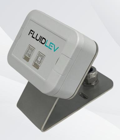
The FLUIDLEV is a fully assembled LoRa drop in tank ATG solution for diesel, oil and AdBlue tanks. Options of 3, 6 or 10m probes 0-3m depth LoRa module allows it to connect directly to an AFM or MICRO FMS system with a Comslink communication module fitted or to any of our Fluidlink Gateway-compatible devices. It is designed to be installed in minutes and has a magnetic key to activate the unit. It is also supplied with a spanner to aid in quick installation.
