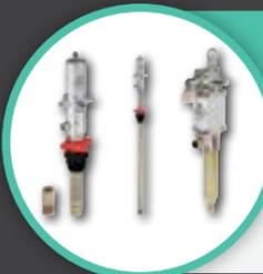
Designed and manufactured in Italy for pumping a wide range of oils. The double-action of RAASM pumps is obtained with solutions that have simplified the pump mechanism itself, ensuring that delivery of the fluid in both alternating movements (upstroke and downstroke) of the pump occurs only through the difference in volume between the diameters of the pumping piston.
